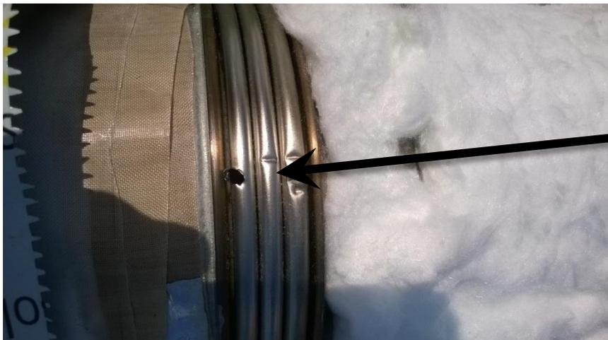
***After more than 20 freezing and thawing cycles vacuum has been intentionally broken***
